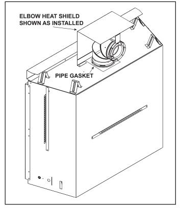
Figure 9.2 Elbow Shield Shown Installed
